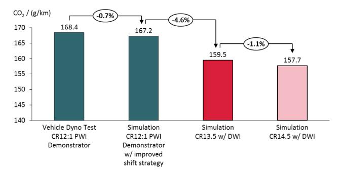
Waterfall diagram for  $CO_2$  emission results in the WLTC-H. The first bar on the lefthand side complies to result from dynamometer testing, the following two bars are results from longitudinal engine simulation using engine map data from the engine dynamometer. The last bar, on the righthand side, shows a result from longitudinal engine simulation with a further engine map scaling to higher compression ratio 14.5:1.
